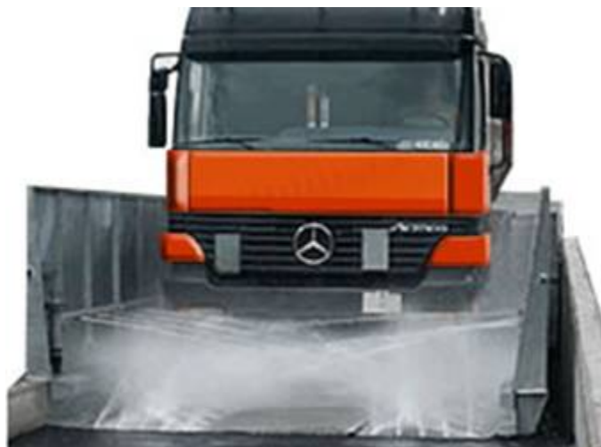
Figure 1: Example of a Wheel Washing System
